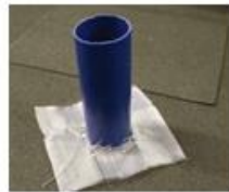
Joint tape cut around pipe
